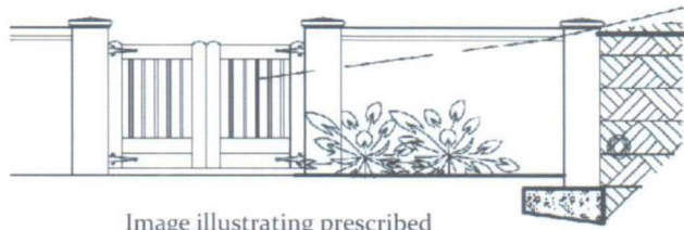
Image illustrating prescribed retaining wall at 1.50m high.
